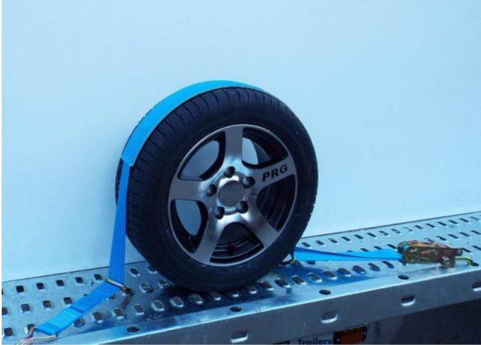
The ends of the over wheel strap must be hooked into the chassis frame of the trailer (not the punched decking) then the diverter hooks are position forward and rear of each individual wheel. **Thread the strap through the ratchet head and pull all of the slack through the head before tightening the strap with the ratchet head.**
