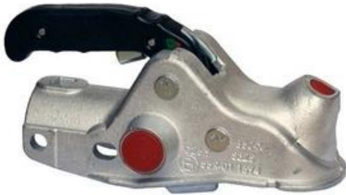
Alko AK301 head, Lift the black handle before coupling the trailer, Handle will snap closed. Red indicator on the front will show Green when coupled correctly.
