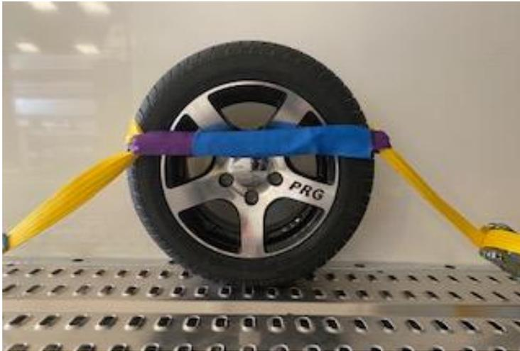
You must make sure that the soft loop strap is positioned 2/3<sup>rd</sup>'s of the way up the wheel, If the strap is too high there will be a chance that it can slip off the top of the tyre, if it is too low the strap can fall down and become loose. **Thread the strap through the ratchet head and pull all of the slack through the head before tightening the strap with the ratchet head.**
