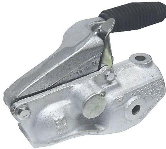
Alko / Bradley coupling head, Using your thumb pull the silver catch backwards and lift the handle, this will then stay in the open position. It will snap closed when correctly coupled.
